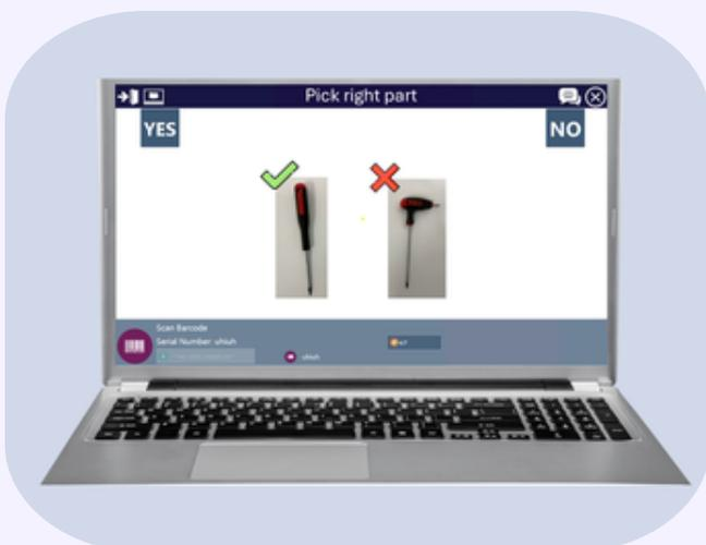
Digital work instructions are interactive, often visual, step-by-step instructions delivered through pc screen. They break down complex tasks into manageable steps, providing visual cues, guidance, and checks that make it easier for operators to complete their work correctly and efficiently.
